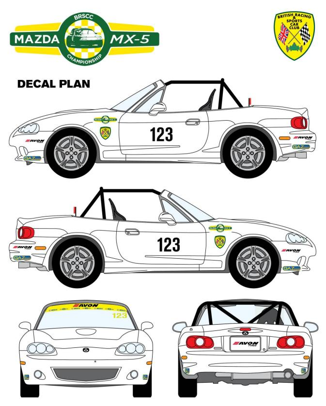
The yellow championship screen visor must be displayed at all race meetings. Race numbers for the windscreen, and small ones for the section of the roll cage behind the drivers head, will be provided by the BRSCC. The Championship, BRSCC and Gaz logos to be placed on the car as per the diagram. The Avonrear number plate decal is available as a rectangle version for Eunos and the long version for UK cars.
