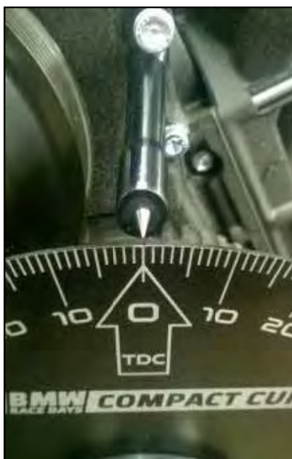
*4. Indicator positioned on Timing Disc according to deadstop readings.
