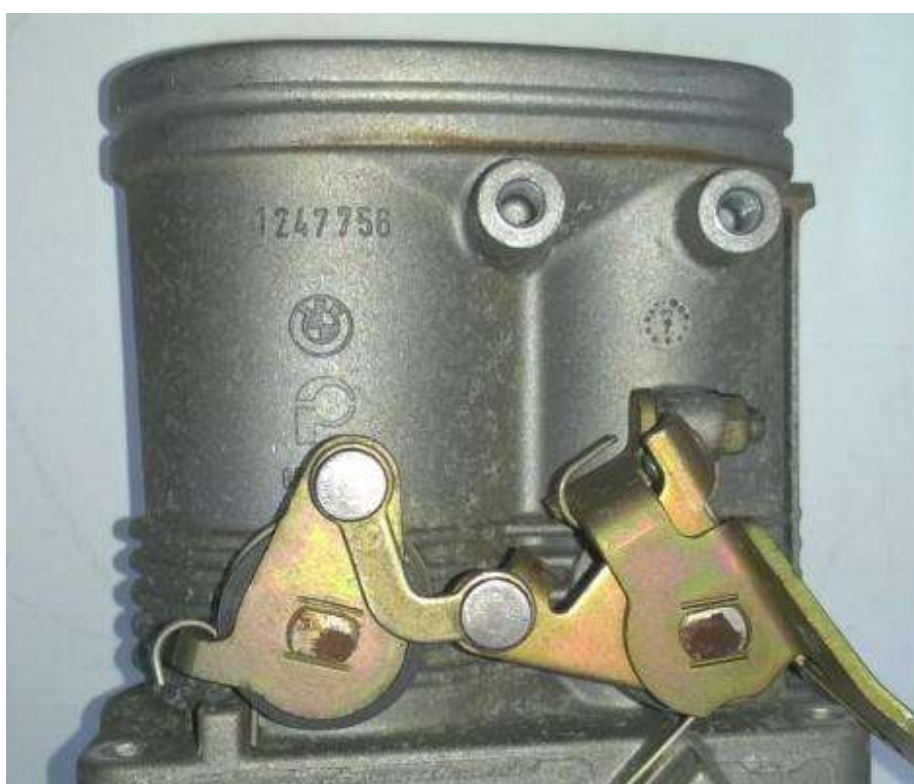
Standard Part Throttle Body showing casting numbers & butterfly linkage. All of which must remain unaltered.
