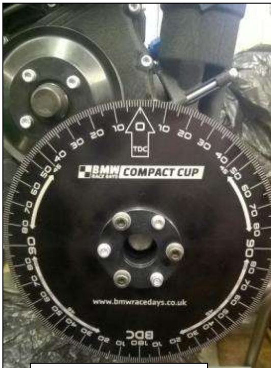
*2 Degree Wheel Installed
