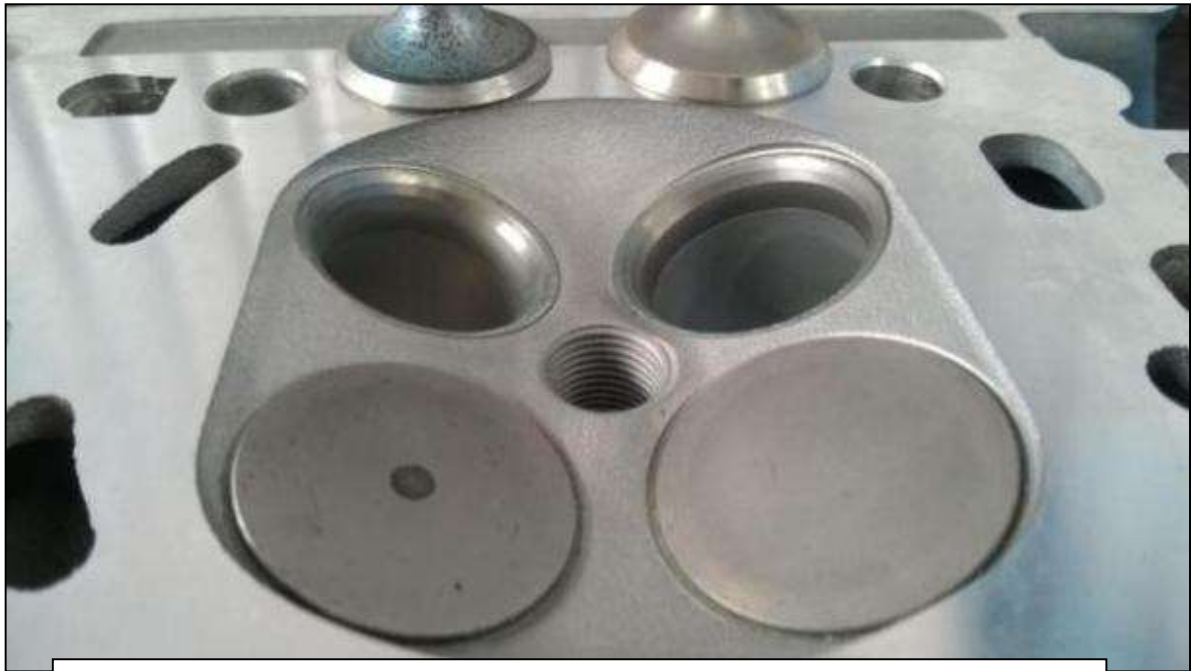
Combustion chamber showing OEM standard installation of valve seats. OEM standard part or standard pattern valve seats must retain the original OEM standard part dimensions and seat angles.
