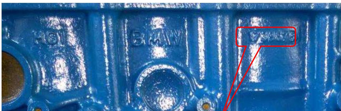
Casting number on M44 block. (typical)
