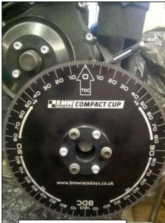
*2 Degree Wheel Installed
