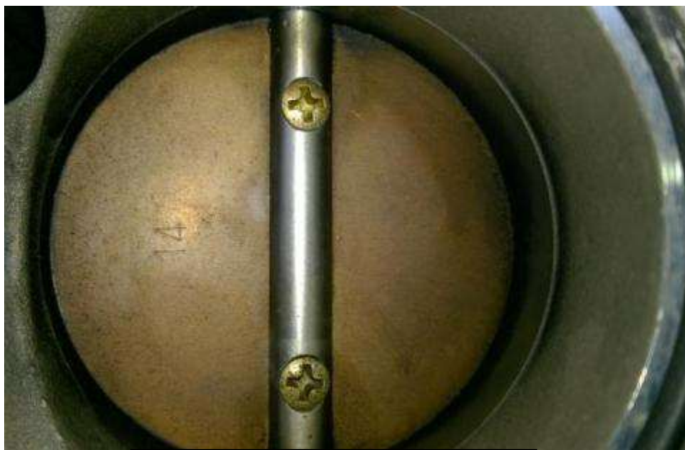
Detail of throttle body spindle (secondary)
