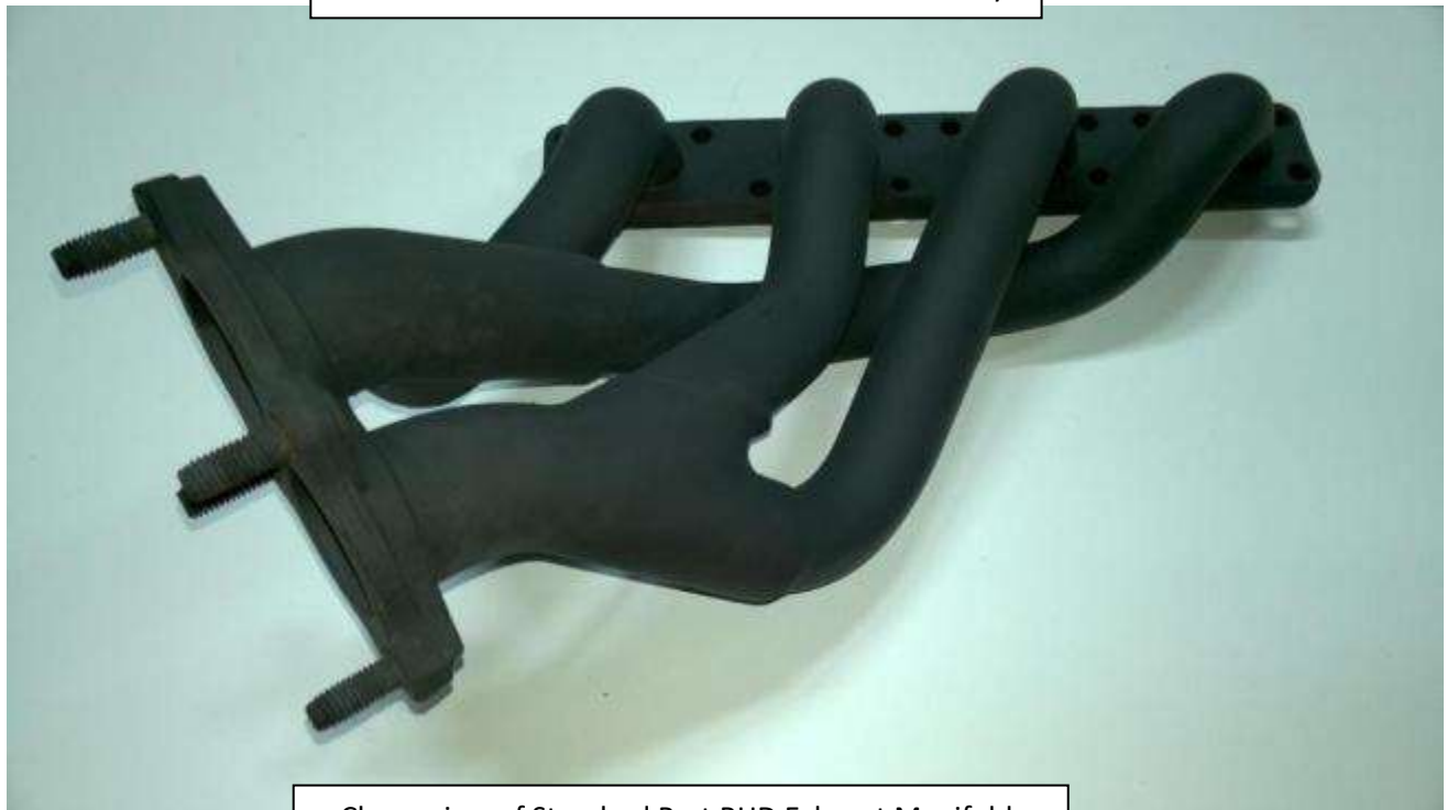
Closer view of Standard Part RHD Exhaust Manifold.
