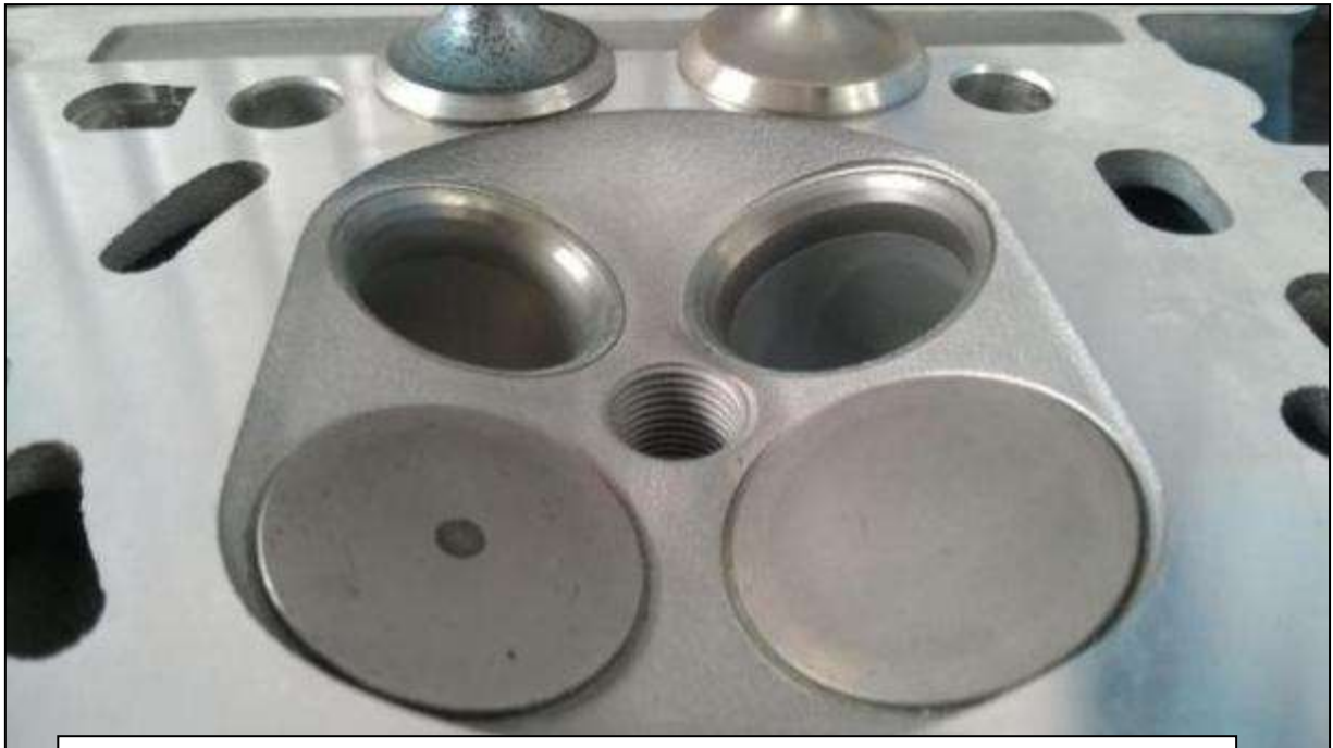
Combustion chamber showing OEM standard installation of valve seats. OEM standard part or standard pattern valve seats must retain the original OEM standard part dimensions and seat angles.
