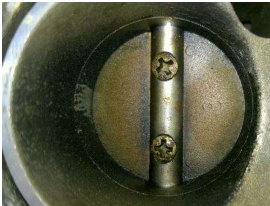
Detail of throttle body spindle (primary)
