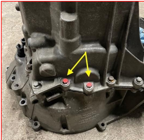
Photo 2 – Gearbox specified bolts
