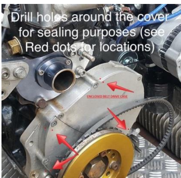
'Sealing 10' – Timing cover, belt drive
