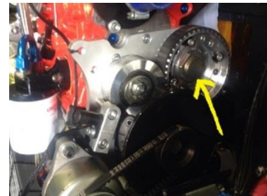
'Sealing 6' – Camshaft end nut
