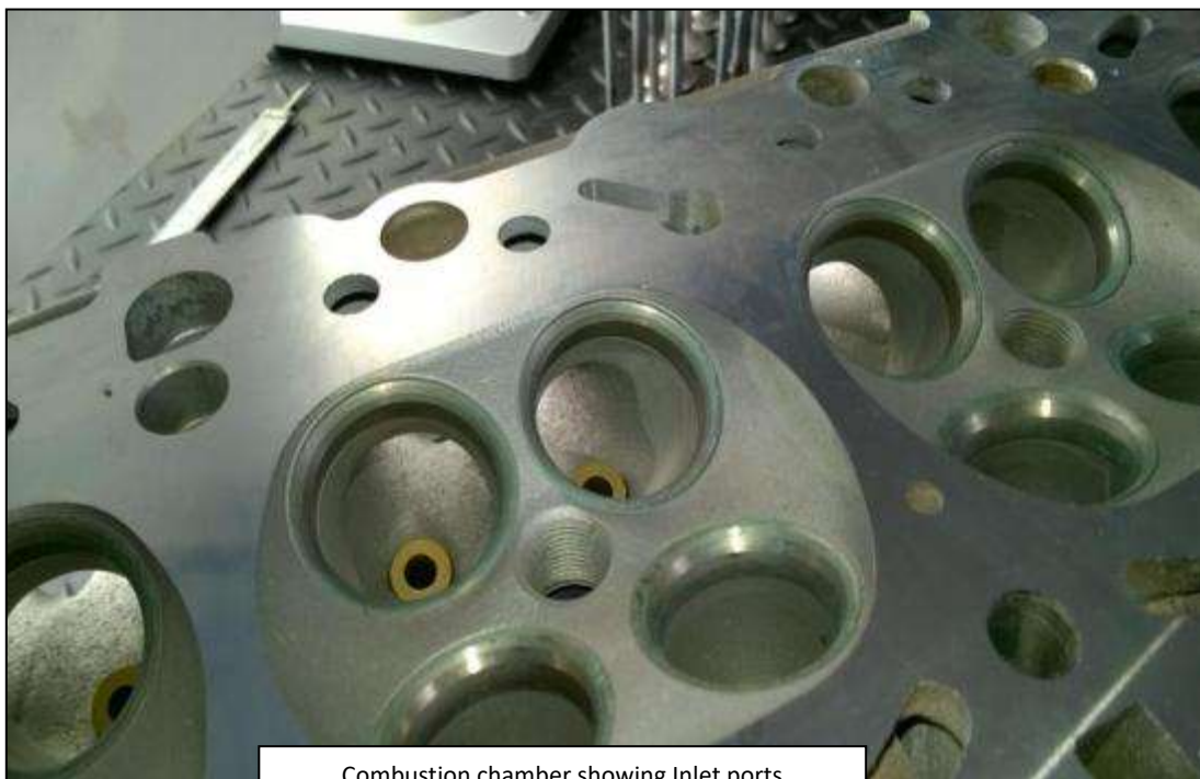
Combustion chamber showing Inlet ports with typical 'as cast' finish
