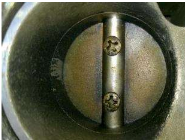
Detail of throttle body spindle (primary)
