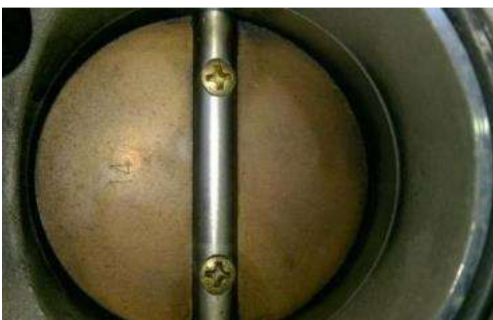
Detail of throttle body spindle (secondary)
