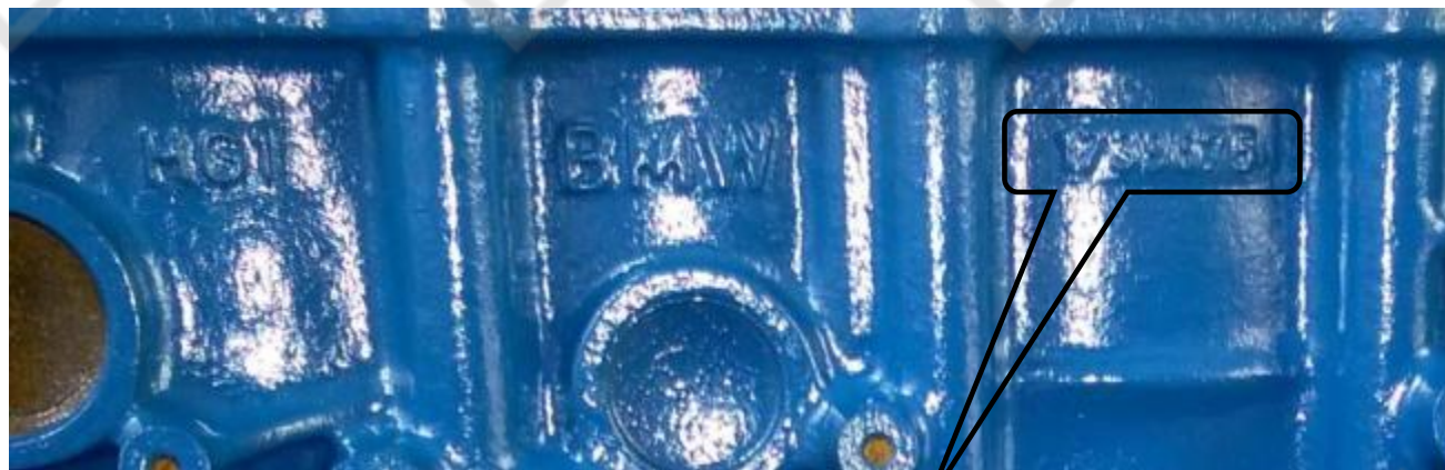
Casting number on M44 block. (typical)
