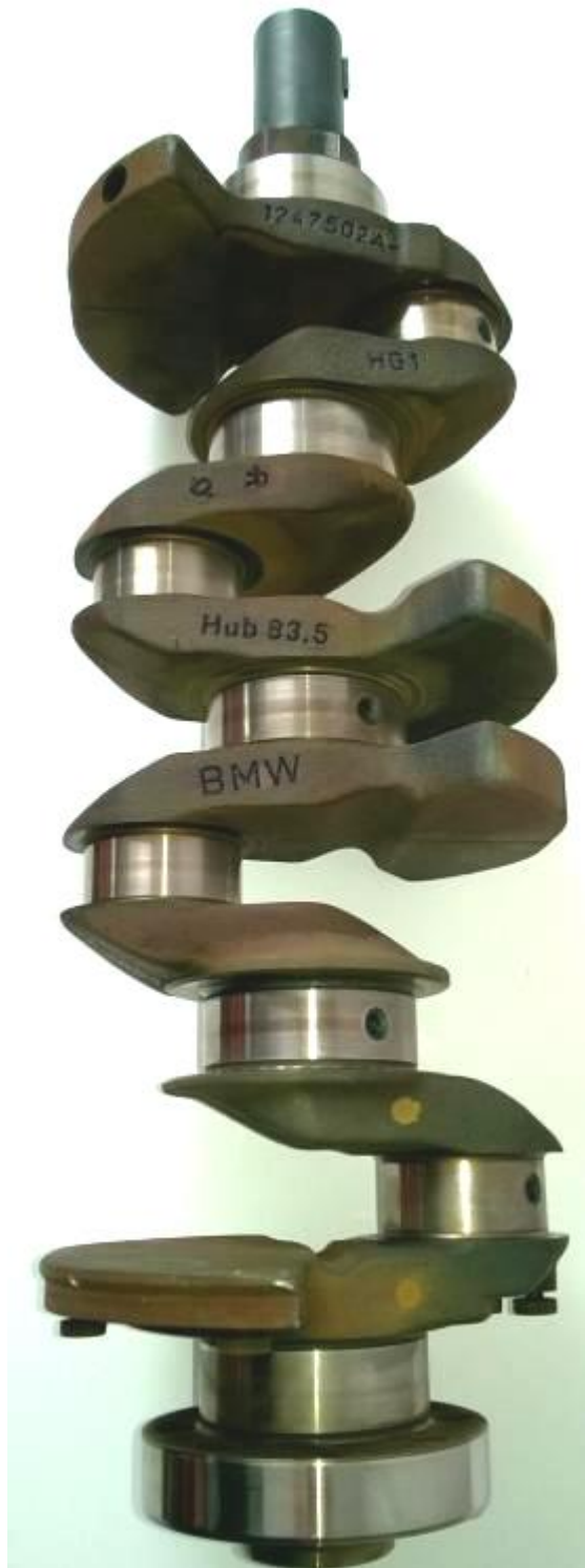
Standard Part Crankshaft showing casting number and stroke (Hub 83.5)
