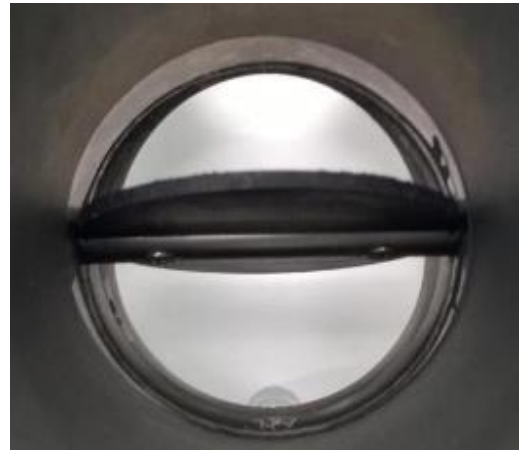
Position of secondary butterfly at W.O.T. showing over Centre rotation. This positioning must not be adjusted from the Standard Part OEM setting.
