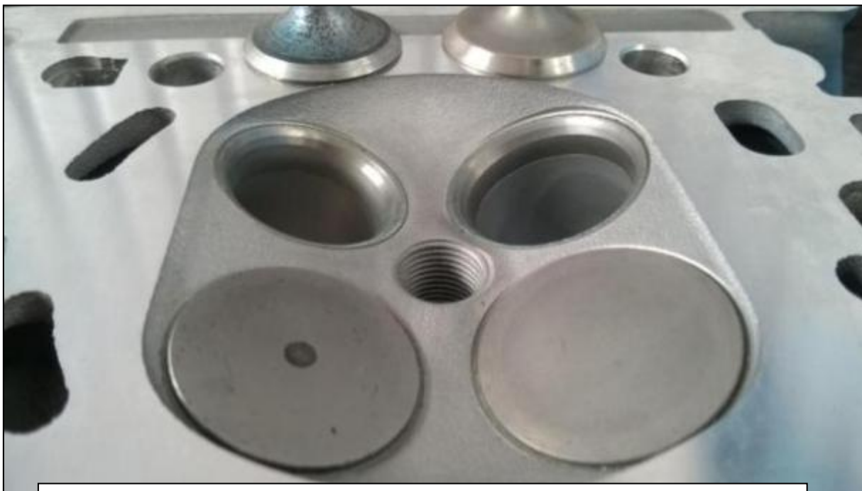
Combustion chamber showing OEM standard installation of valve seats.
