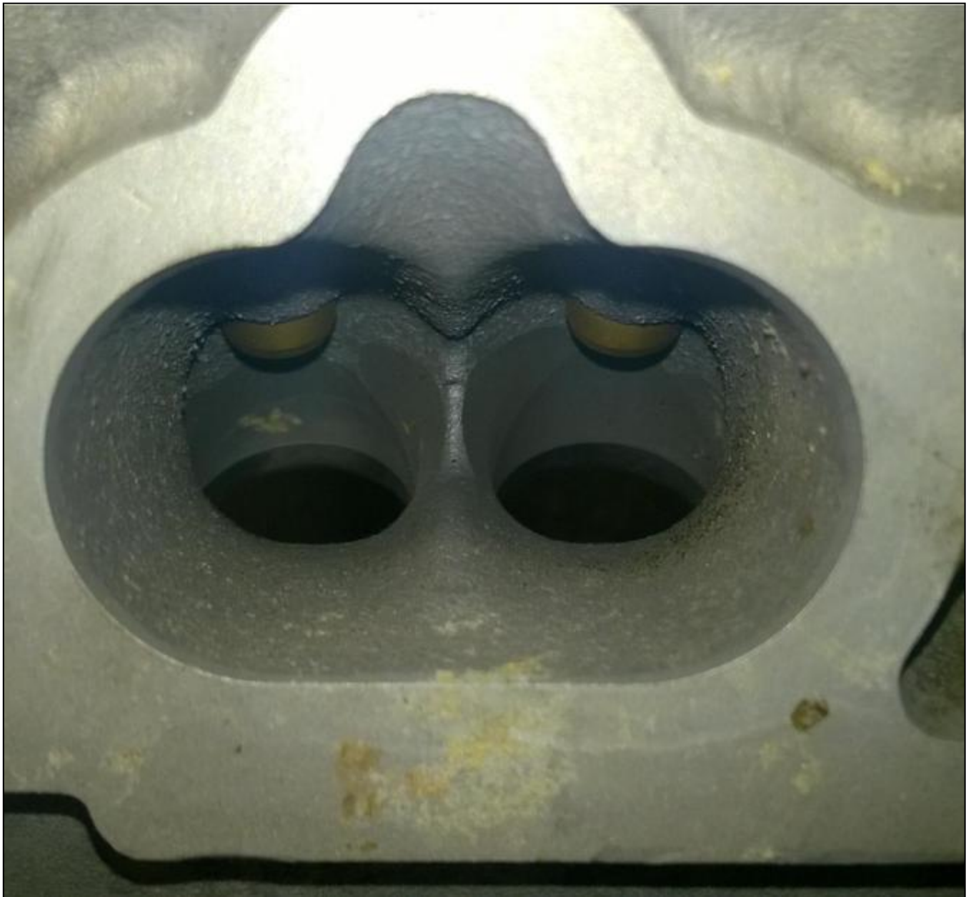
Intake port showing OEM standard part machined area under valve seat & 'as cast' surface finish extending up to the machined area of port (typical).
