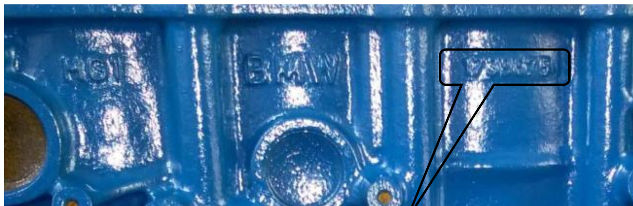
Casting number on M44 block. (typical)
