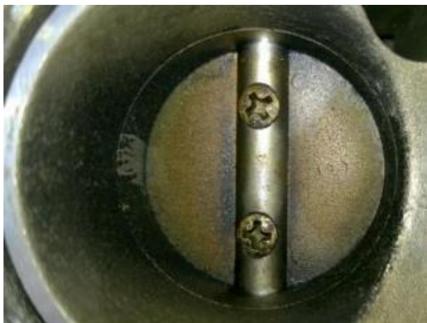
Detail of throttle body spindle (primary)
