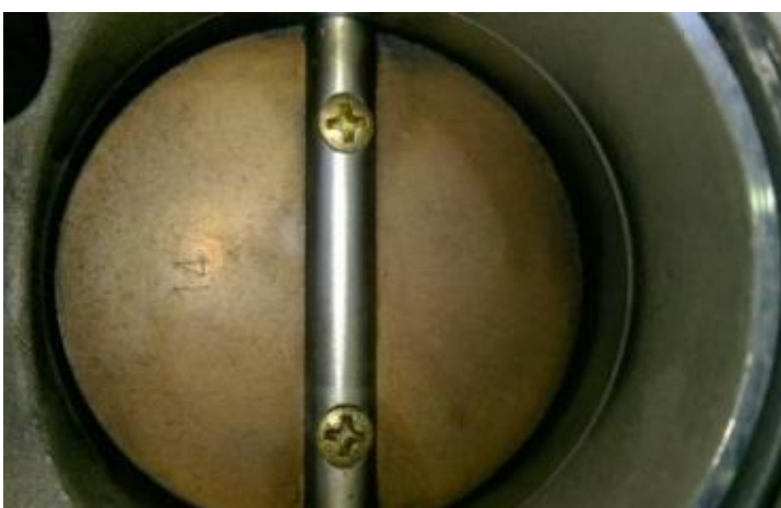
Detail of throttle body spindle (secondary)
