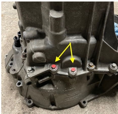
Photo 2 – Gearbox specified bolts
