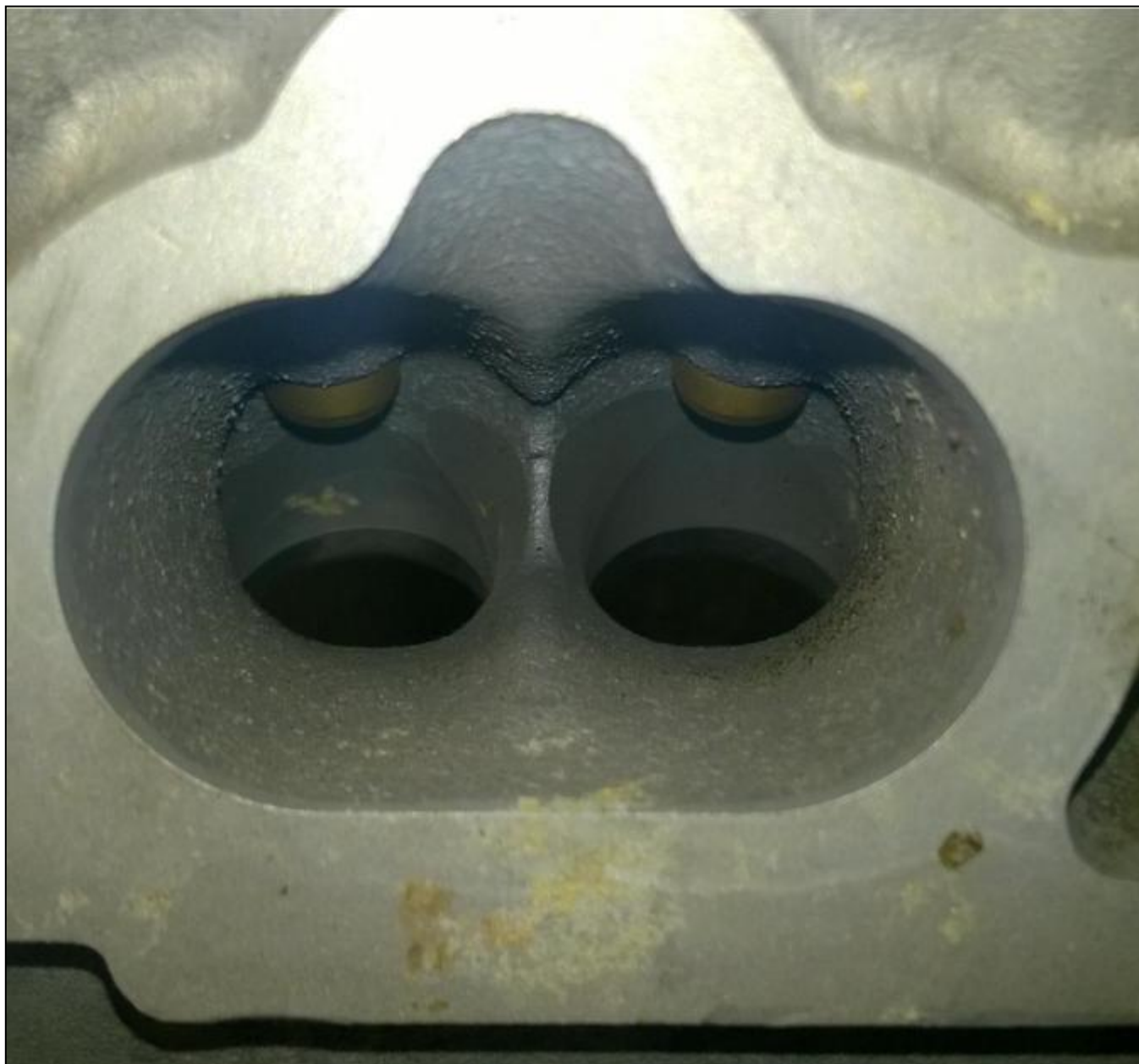
Intake port showing OEM standard part machined area under valve seat & 'as cast' surface finish extending up to the machined area of port (typical).
