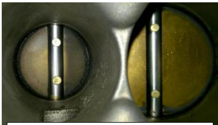
Detail of throttle body spindles & locked screw fittings.
