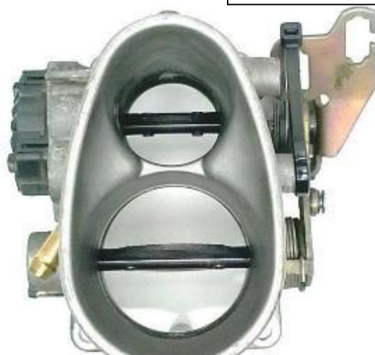
Position of secondary butterfly at W.O.T. showing over Centre rotation. This positioning must not be adjusted from the Standard Part OEM setting.
