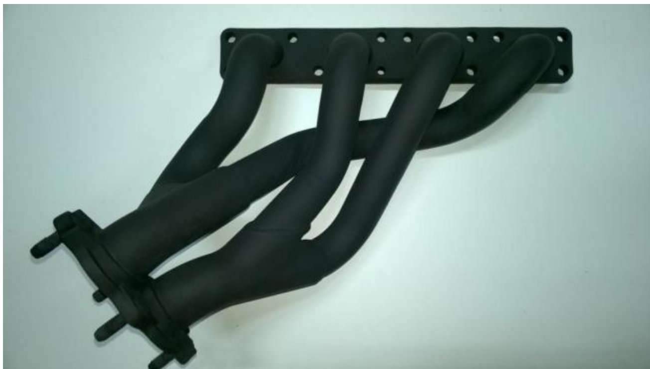
Standard Part RHD Exhaust Manifold is mandatory
