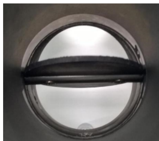
Position of secondary butterfly at W.O.T. showing over Centre rotation. This positioning must not be adjusted from the Standard Part OEM setting.
