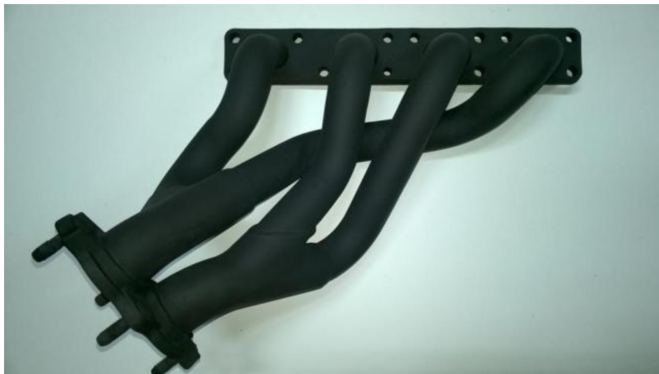
Standard Part RHD Exhaust Manifold is mandatory
